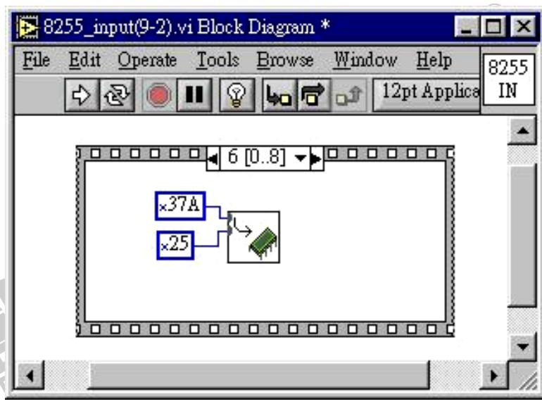
10、At the eighth page frame please add this step as follows. When we send /RD as low level voltage, 8255 will put the data of indicated PORT on the data bus of 8255. So, this program read directly the data from the parallel data bus. (Because of those data bus are connected together).
