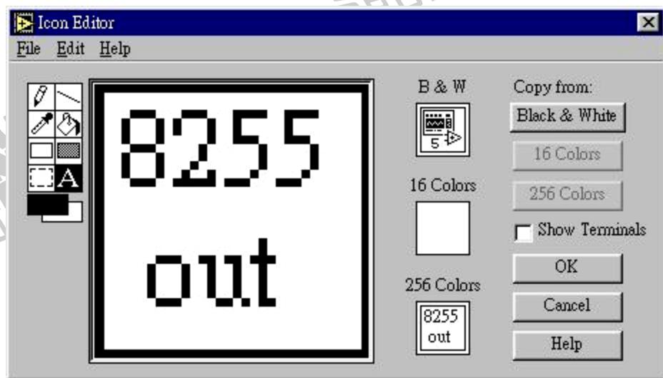
16、You can see the graphic picture on the right upon corner has changed. Now, we need to define which control element should be pulling out from the subprogram. Please click right button on the graphic interface upon the window. Then choose "**Show Connector**", you can find the graphic picture is dissevered into two parts, just like picture No. 2.
