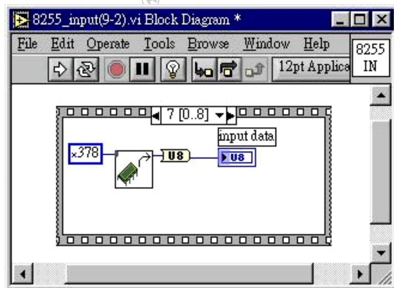
11、At the ninth page frame please add this step as follows. This action is to send /RD signal as high level voltage. It means to stop reading external data.
