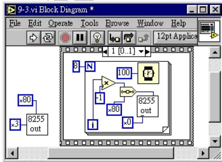
Continuous Run Button 8、Press Continuous Run Button to watch whether the LED rolling control
