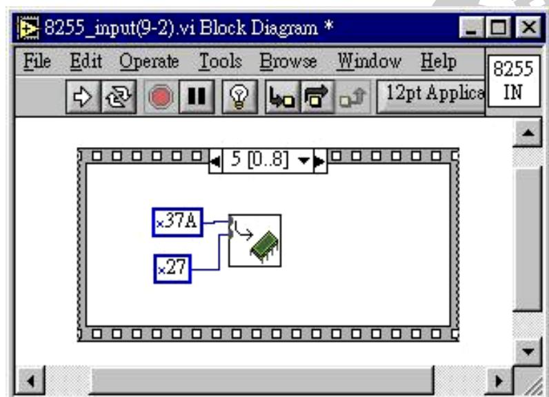
9、At the seventh page frame please add this step as follows. This step is how to send /RD signal as low level voltage and informs 8255 for reading external data.
