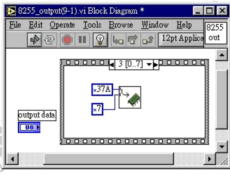
9、At the fifth page frame please add this step as follows. This step is how to send data. For example, if we want sending data to PORT A. Firstly, set the address as 00h, then sending data to PORT A of 8255. Another case if we want setting the control word register of 8255 and three PORTs as output, then the address should be set as 03h and output data should be 80h.
