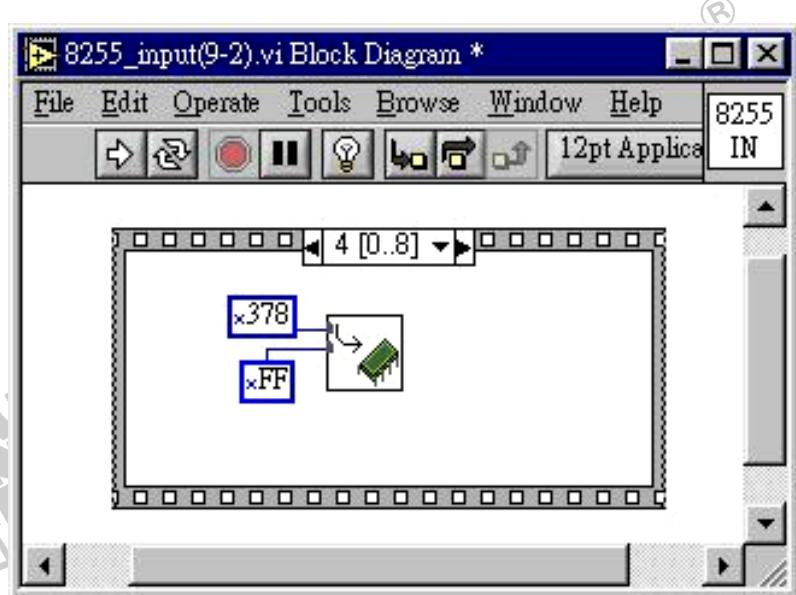
8、At the sixth page frame please add this step as follows. This step is how to set 8 bits data bus of parallel port as data input.
