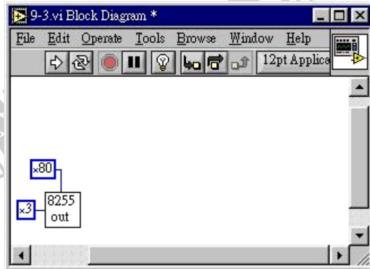
3. Select **“Functions> All Functions>Structures>Stacked Sequence Structured”**. Pull out one block to make it two new frames. Make the first frame to be connected as the following program. It means sending the first value as 80h. High bit LED output is high level voltage (LED on), the others are low level voltage (LED off).
