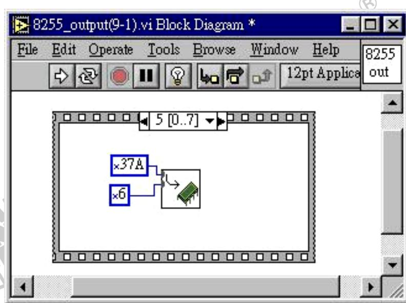
11、At the seventh page frame please add this step as follows. This step is how to delay 1 msec. It means /WR of 8255 has to be written during the specified time, so the data could be received correctly.
