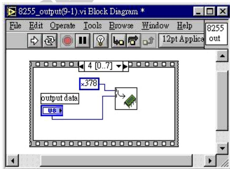
10、At the sixth page frame please add this step as follows. This step is how to set /WR as low level voltage. It means to inform 8255 for data input.
