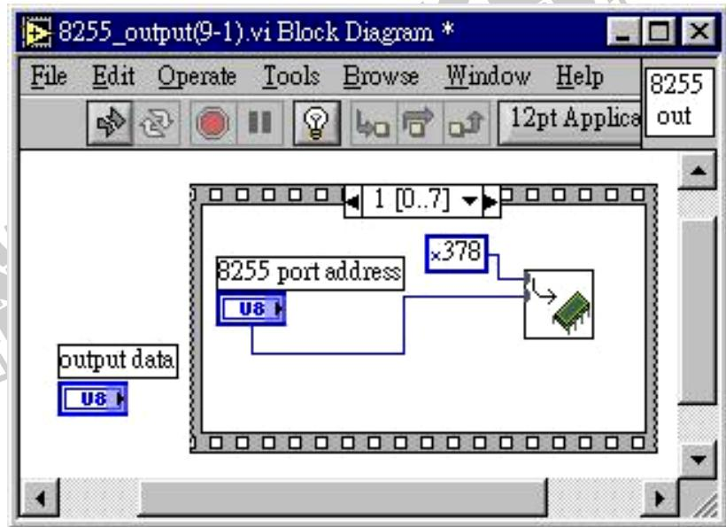
7、At the third page frame please add these steps as follows. Those steps are how to set ALE of 8255 as high level voltage. It means to use 74373 IC to latch the sending address.
