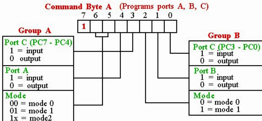
Someone may ask where is the address of the control word register of 8255. There must be some specified address that pointed to those register. Sure, memory management distributes four address pointed to the registers of 8255, that is **00h assigned to PORT A, 01h assigned to PORT B, 02h assigned to PORT C, and 03h assigned to the control word register**. Due to one single chip 8255 we use, so we don't need any decoder to expand the address. But in
